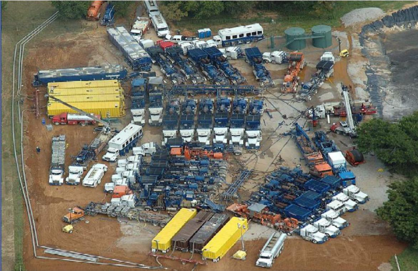
Apache Horn River 10-frac: 2.4 million kg sand; 32 million Lts water.....
